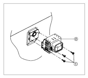
**CAUTION**: Never install the magnetron without the metallic gasket plate which is packed with each magnetron to prevent microwave leakage. Whenever repair work is carried out on magnetron, check the microwave leakage. It shall not exceed 4mW/cm² for a fully assembled oven with door normally closed.
